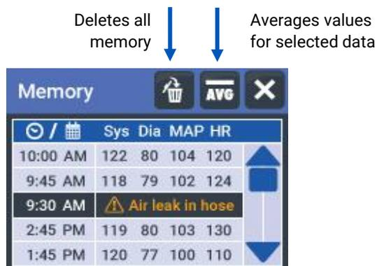
To view previous readings, touch Menu, then touch the Memory icon. Select the parameters to view. The time and date will alternate. Up to 960 measurements can be stored in memory.
